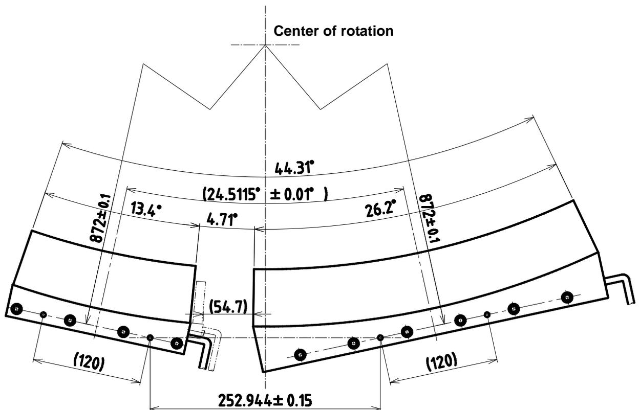
Figure 7. Orientation of the CL units (when the two CL units are connected)
