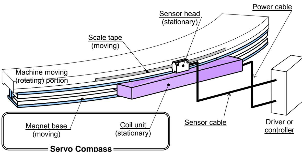
Figure 1. System configuration
