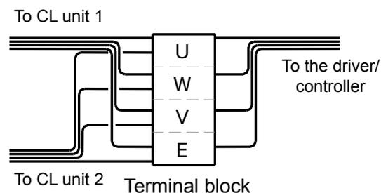
Figure 6c. Connection terminal block wiring specifications
