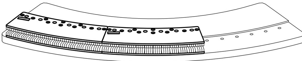
Figure 5c. Connecting MG bases
