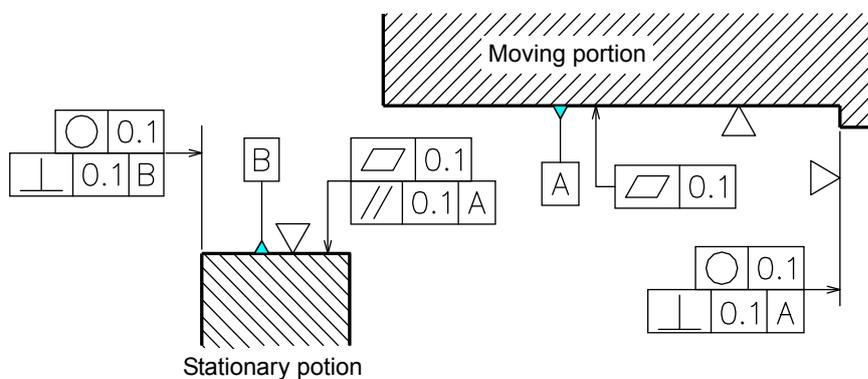
Figure 3b2. Recommended surface accuracy
