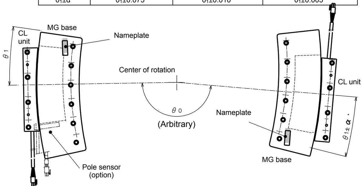
Figure 9a. Relative position relationship between MG bases and CL units
