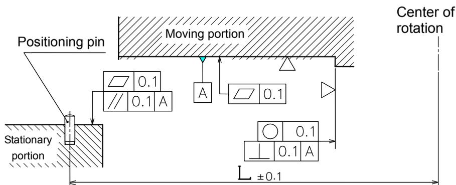
Figure 3a2. Recommended surface accuracy
