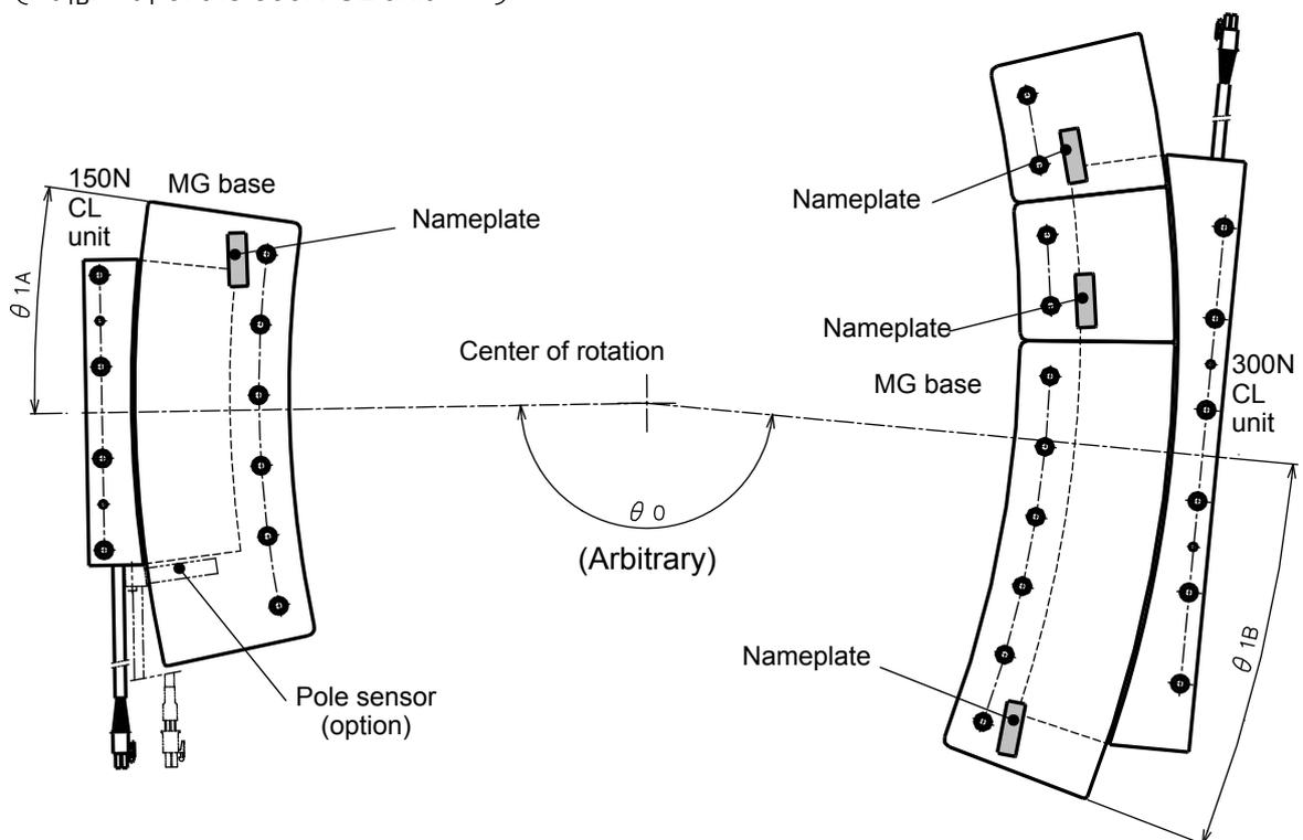
Figure 9b. Relative position relationship between MG bases and CL units
