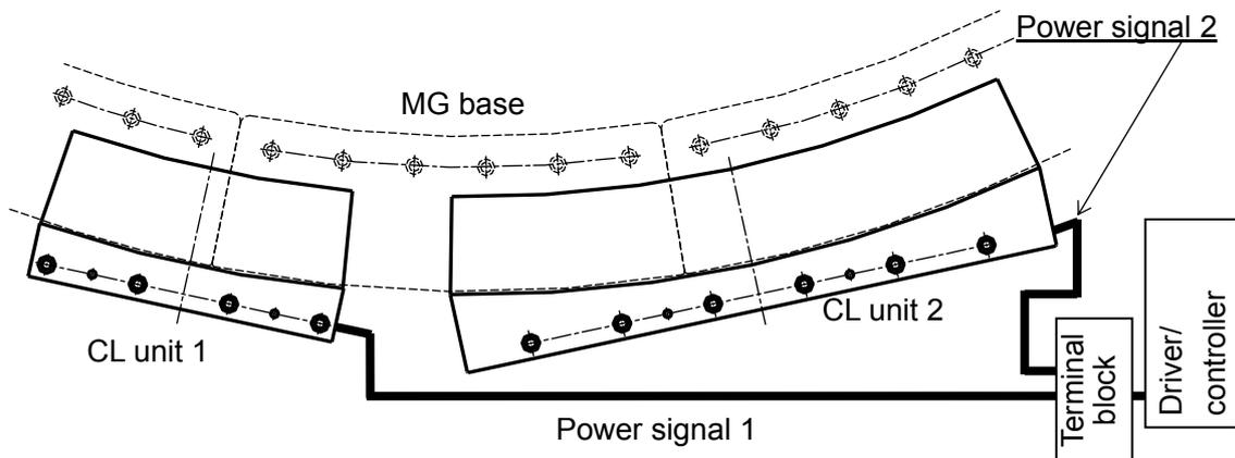
Figure 6a. CL unit wiring (for adjacent mounting)
