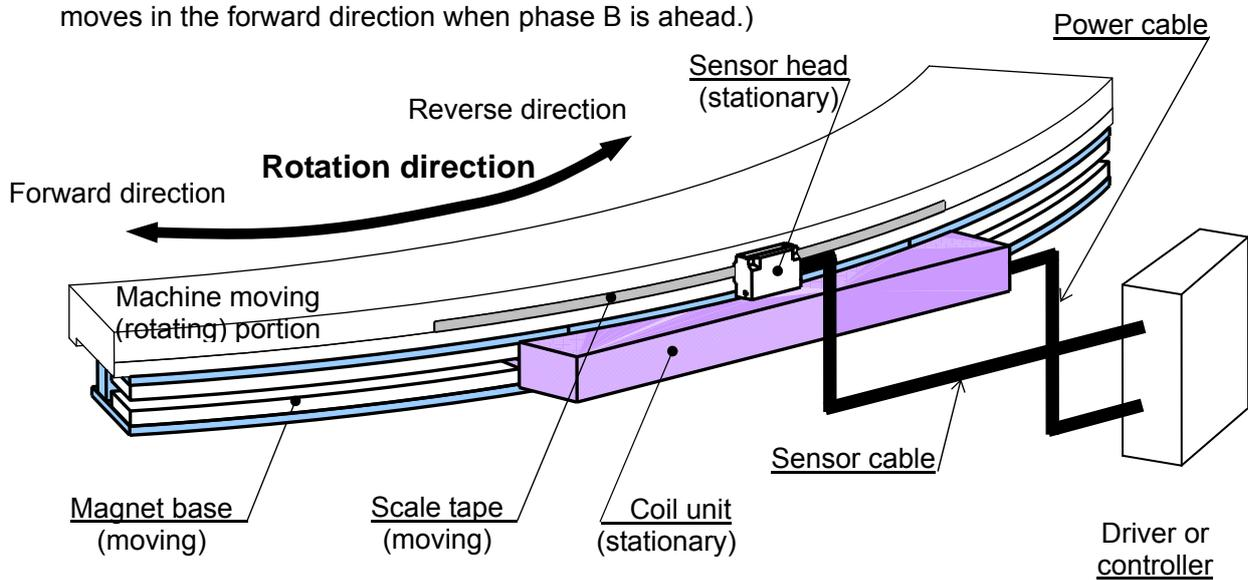
Figure 2. Rotation directions of the Servo Compass
